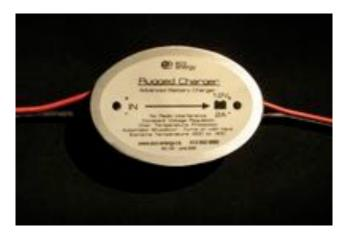
The rugged 12V charger, keeps refrigeration unit batteries charged by taking a trickle charge from the trucks wiring harness and transferring it to the refrigeration unit, or to charge GPS trackers.
