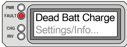
**Dead Battery Charge** appears on the LCD and the FAULT (red) LED is on. The PWR (green), CHG (green) and INV (green) LED's are off.
