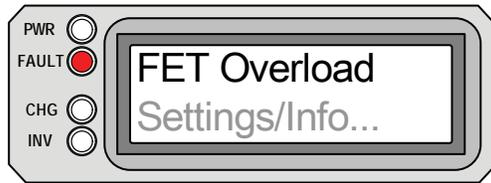
**FET Overload** appears on the LCD and the FAULT (red) LED is on. The PWR (green), CHG (green) and INV (green) LED's are off.
