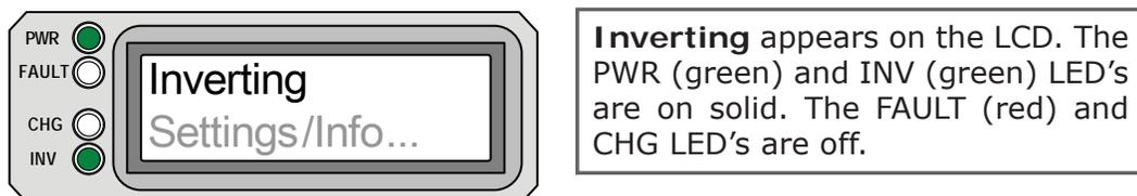
**Figure 5-4, Inverting Mode**
