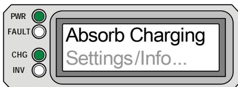
**Absorb Charging** appears on LCD; PWR (green) is on solid and CHG (green) LED is typically on solid, but may blink slowly; FAULT (red) LED is off and INV (green) LED could be on or off.
