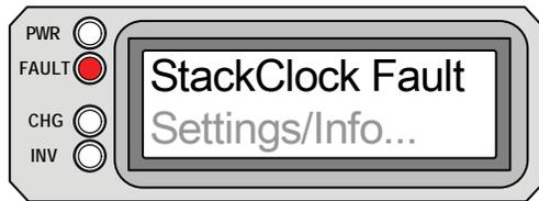
**StackClock Fault** appears on the LCD and the FAULT (red) LED is on. The PWR (green), CHG (green) and INV (green) LED's are off.
