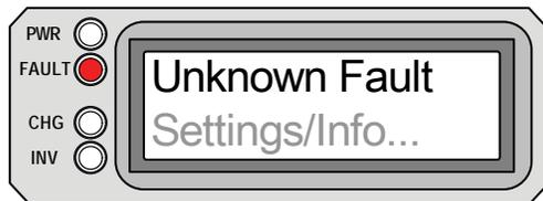
**Unknown Fault** appears on the LCD and the FAULT (red) LED is on. The PWR (green), CHG (green) and INV (green) LED's are off.
