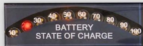
Batteries have only a 20% charge
