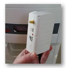
Regardless if it's BlueTooth, WiFi or ZigBee, the hardest part of any wireless communication setup is getting it going. For this trick you might need an extension cord to get power to the Home Gateway where the inverter is located, but the success rate is almost 100%.
