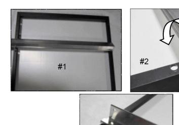
**For T-Slot Rails**: Lay T-Slot rails across the short axis of the panel as shown in Photo #1. Slide stainless bolts into T-slot of rail and position so they are opposite to the mounting holes on the frame
