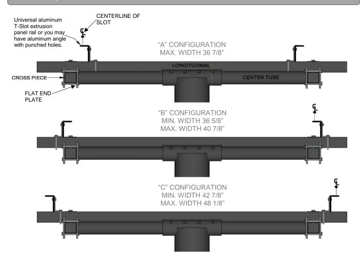
To determine which configuration to use for your modules, measure center of hole to center of hole on the LONG edge of module (see drawing below). These are the holes that you will use to fasten to the slots in the rails shown. Compare this dimension to dimensions shown above and choose the most advantageous configuration.
