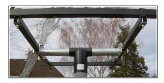
Attach aluminum angle brackets to longitudinals with square U-bolts. Oppose angle brackets so they face in toward each other. Attach aluminum rails (see detail on page 6).
