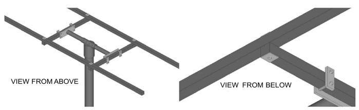
Place longitudinal tubes on top of cross pieces and bolt with square washers top and bottom.
