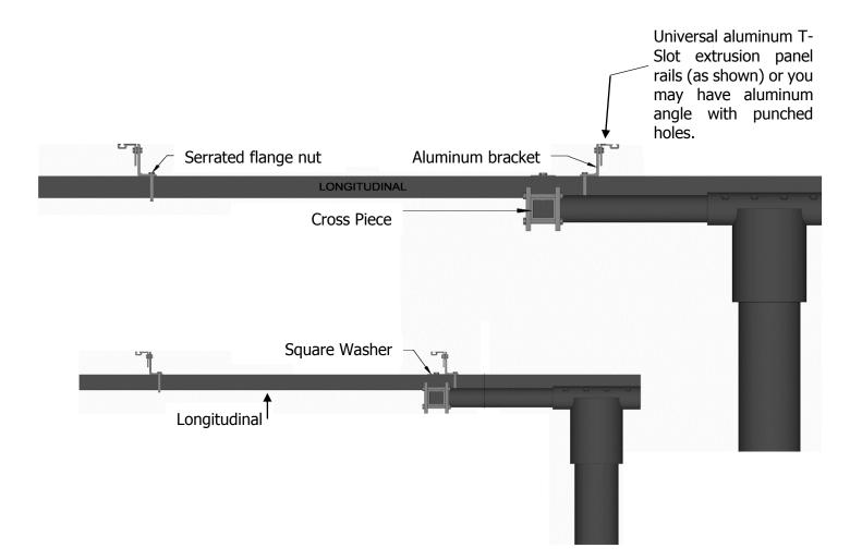
Bracket orientation in most installations is generally opposed to one another as in top picture. It may be necessary to have brackets facing in same direction as in bottom picture, if panel size is such that you need to do this to maintain a  $\frac{1}{4}$  gap between panel ends on centerline.
