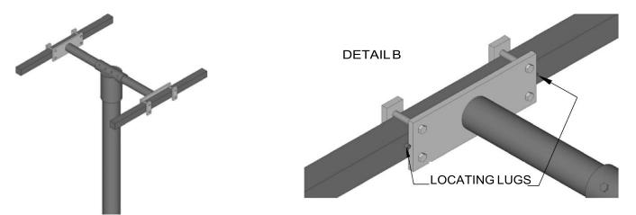
Slide cross pieces into U-Bolts or bolt and flat bar arrangement. Make sure locating lugs on cross pieces are facing in. See Detail "B" of locating lugs.
