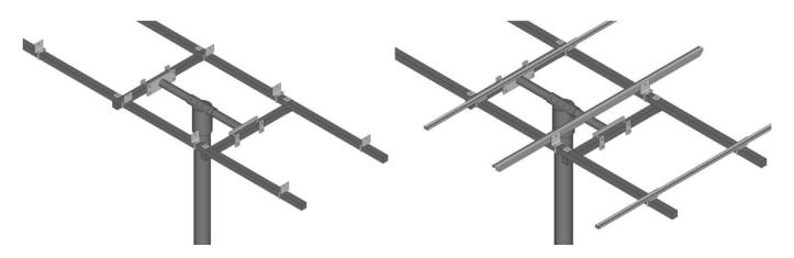
Attach aluminum angle brackets to longitudinals with smaller square U-Bolts and whiz flange nuts. Oppose aluminum angle brackets as shown. Some mounts come with aluminum angle with punched holes for bolting on panels, and some come with aluminum extrusions which allow for panel attachment bolts or clips to slide in the "t-slot".
