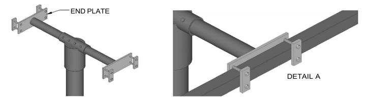
Finger tighten onto "Tee" end plates, either the U-Bolts or aluminum flat bar and straight 1/2" bolts, whichever come with your mount. Place entire "Tee" assembly on top of post. The aluminum flat bar and straight 1/2" bolts are shown in Detail "A".
