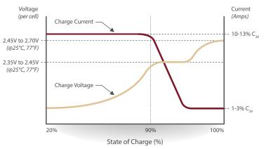
Note: Charging time will vary depending on battery size, charger output, and depth of discharge.
