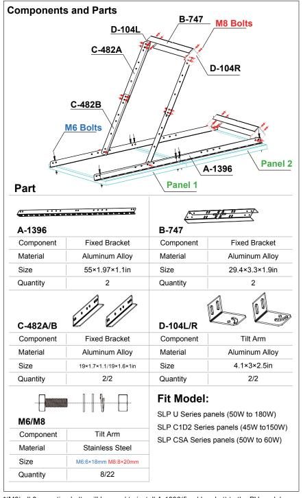
\*(M6) all 8 mounting bolts will be used to install A-1396(fixed bracket) to the PV module frame. Place 1 mounting bolt on each corner of the PV module frame.
