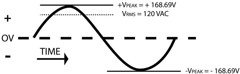
Fig. 5.1: 120 VAC, 60 Hz Pure Sine Waveform
