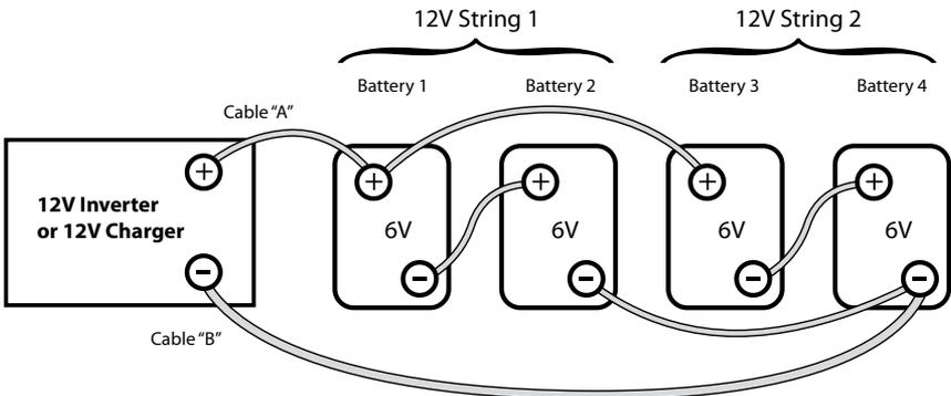
Fig. 7.4: Series-Parallel Connection
