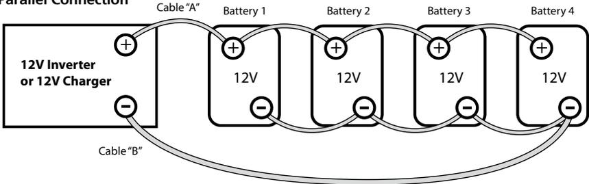
Fig 7.3: Parallel Connection
