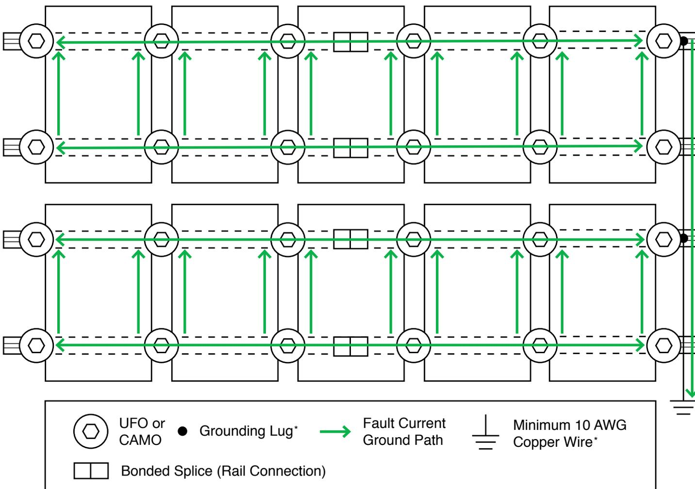
\*Grounding Lugs and wire are not required in systems using certain Enphase microinverters or certain Sunpower modules. Equipment grounding is achieved with the Engage cable for Enphase or the AC module cable system for Sunpower via their integrated EGC.
