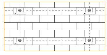
Tighten S-5! M10 bolt to 240 in-lbs or S-5! Mini M8 bolt to 160 in-lbs. Use the following fastening guidelines for other S-5! roof clamps: ProteaBracket™ - firmly seat roof screws and tighten hinge bolt to 225 in-lbs; RibBracket™ - firmly seat roof screws and tighten M8 bolt (M8-1.25 x 22mm sold separately) to 160 in-lbs; and SolarFoot™ - firmly seat roof screws and tighten M8 flange nut to 160 in-lbs.
