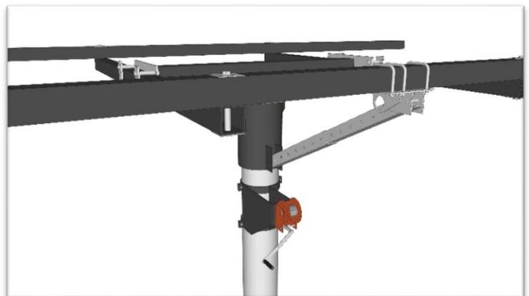
Fully tighten collar on quick link. Pull tension on cable as it comes off winch drum and cut zip ties. Take up slack in cable by turning winch handle while still holding tension on cable. This will prevent it from jamming in winch drum.
