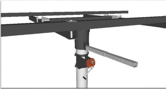
Install the 2 ¼" x 2 ¼" end of telestrut between the lugs on the bottom of the pivot cap. Tighten the nyloc nut all the way.
