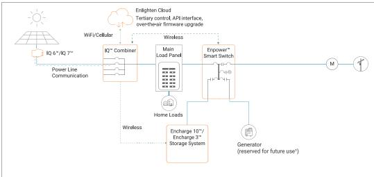
Partial home backup with main load panel as service entrance and PV combiner connected to Enpower. When PV circuits breaker size is less than 80A, this is the preferred configuration for partial home backup with subpanel.
