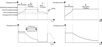
Fig. 1-5 SLD Battery charging stages diagram
