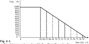
When the ambient temperature rises higher than the set value, the controller will stop charging and discharging.
