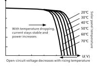
Fig. 1-4 Relation between solar panel output characteristics and temperature
