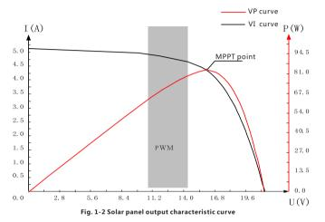
Meanwhile, due to changing ambient temperature and illumination conditions, the max. power point varies frequently, and our MPPT controller can adjust parameter settings according to the environmental conditions in real time, so as to always keep the system close to the max. operating point. The whole process is entirely automatic without the need of human intervention.
