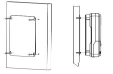
Fig. 2.2 Wall mounting the controller
