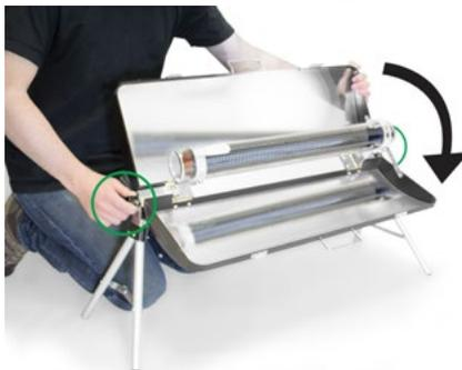
There is a knob at each end of the cooker. Loosen these by a couple of turns to be able to turn the reflectors. Once they are at the desired angle (see next step), re-tighten the knobs.
