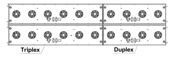
**Step 2:** Use the accessory C\*16PCS to lock the accessory I\*4PCS to the rear mounting holes of the Duplex and Triplex, as the picture shows.
