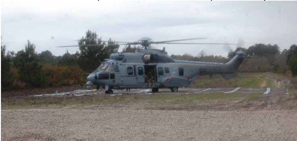
Mobi-Mat® Helipad™ in use with a Super Puma (take-off weight 11,200 kg)
