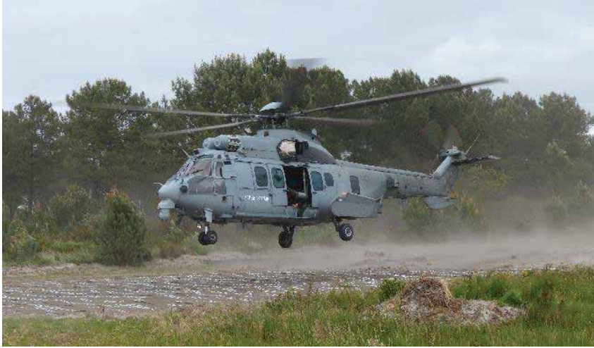
Mobi-Mat® Helipad™ in use with a Super Puma (take-off weight 11,200 kg)
