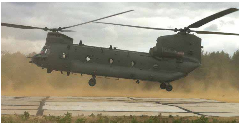
Mobi-Mat® Helipad™ in use with a CH-47 (Chinook) (take-off weight 22,680 kg)
