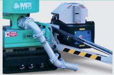
Didascalia di destra: Ø 100 (4") material hose connection manifold, easily removable for machine handling.
