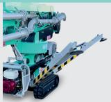
Self-propelled undercarriage on extendable tracks, for easy mobility even on the most uneven terrain.
