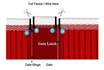
Set Arms "B" and "C" above Arms "A" and "D" so that when the gate opens outward the Arms on the gate ("B" and "C") will pass ABOVE the fence material and Arms ("A" and "D") on either side of the gate. Test opening the gate before you add the Fence material to be sure that the Arms do not hit each other, preventing the gate from opening. Cut the fence between Arms "A" and "B" as well as "C" and "D".
