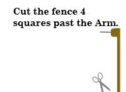
Zip Tie first section to the Arm. Attach second side with Ties and continue installing the fence.
