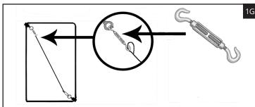
**1G.** Tighten by turning turnbuckle body.
