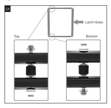
**2A.** Install the hinge hardware as shown for the top and bottom of the gate. Please note: The two black spacers go between the Gate (inner) and Frame (outer).
