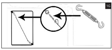
**1G.** Tighten cable by turning turnbuckle body.
