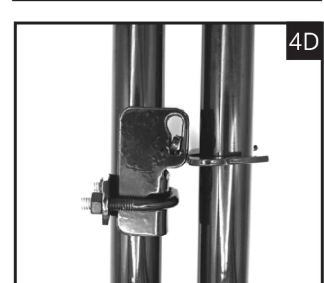
**Step 4.** Use the bolt with the Latch (C) to secure the Latch to Tube (B). The Latch should be oriented to flip up and over the Latch Tube (B) in the open position. When the gate is open, the latch folds upwards flush with the gate frame (4C). See hardware layout for gate latch (4A). Note the orientation of the latch (4B). The two flange drop latch moves up to open (4C) and down to hold the gate closed (4D).
