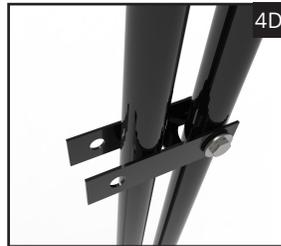
**Step 5.** Slide Male Hinges over the installed post (D). The bottom hinge should point **up** and the top hinge should point **down**. Locate the bottom hinge so that it is 10" from the ground surface and tighten the bolt enough so it stays in place.
