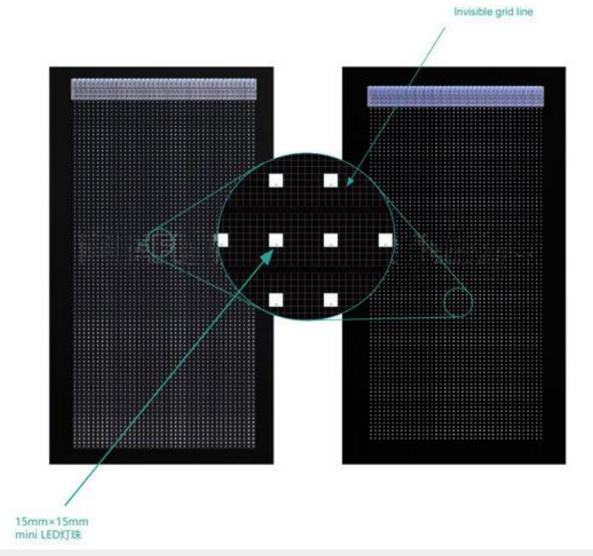
Use the integrated MiniLED lamp beads to improve its own permeability Use invisible grid circuit to improve its permeability
