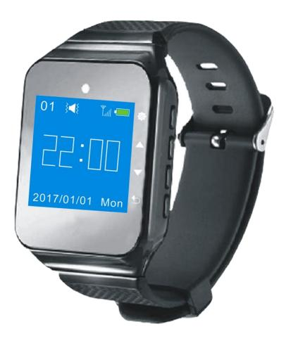
The smart watch pager has a TFT screen display, [ $\bigcirc$ ], [ $\bigcirc$ ], [ $\bigcirc$ ] and [ $\bigcirc$ ] 4 buttons, 1 USB port and 1 LED indicator light.
