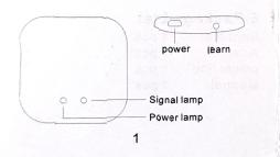
3.3 Delete all transmitters: long press the "learn" setting button for 3 seconds until the blue LED on the right side of the front cover is always on, and then long press the "learn" setting button for 5 seconds after release, until the blue LED light on the right side of the front cover flashes for 4 times, and all transmitters are deleted successfully.
