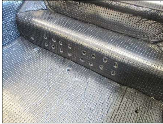
Sound-absorbing coating– Internal lower side
