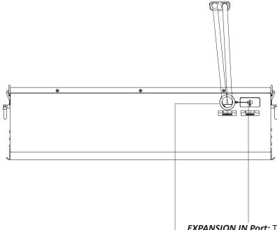
**EXPANSION IN Port:** This port allows Daisy Chain connections.
