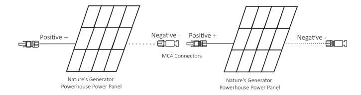
3. Connect the MC4 connectors of your Power Panel Cable to the remaining MC4 connectors on the Nature's Generator Powerhouse Power Panels. A minimum of two serial connected Nature's Generator Powerhouse Power Panels are needed to recharge Nature's Generator Powerhouse Lithium Power Pod.
