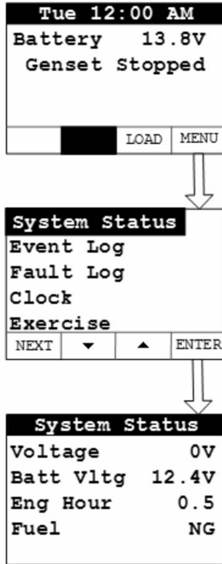
FIGURE 14. SYSTEM STATUS SCREEN
