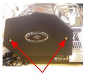
Unscrew 13mm nuts, then Pull panel off machine.
