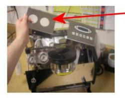
Carefully lift left side of front panel as shown. Be VERY careful NOT to disconnect cables behind the touchpad they are identical. Either set panel aside with cables attached or label them with a marker before disconnecting.
