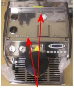
Remove 2 phillips screws Then remove top panel.
