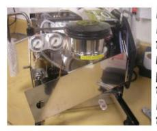
Pull left side of bottom panel forward. You may have to push discharge tube on bottom left of panel up to remove.
