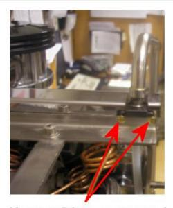
Unscrew 2 brass screws and then remove steam wand from top of machine.
