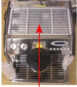
Slide flat blade screwdriver Under cup tray grill and then Gently pry it up to lift it off.
