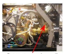
Rotate steam valve until threaded connection is facing straight up.
