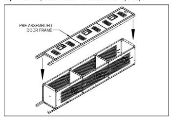
**Step 5:** Tighten all fasteners checking for squareness of the locker while tightening. Attach optional sloping hood, end bases or front base (see pages 4 and 5).
