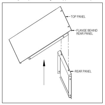
**Step 2:** Assemble the side panels to the top panel and rear panel with #10 - 24 x 3/8" long slot less screws and #10 nuts (provided).
