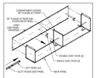
Step 3: Attach the second side panel and the right rear leg to the assembly of Step 2. Attach an additional two single coat hooks to the second side panel. The locker chassis is now complete.
