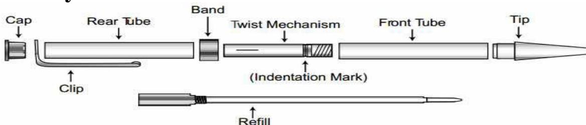
A. Press the tip into the front tube.
