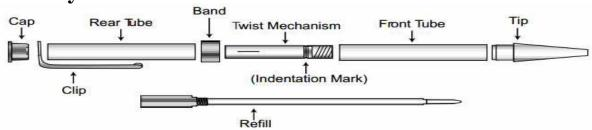
A. Press the tip into the front tube.
