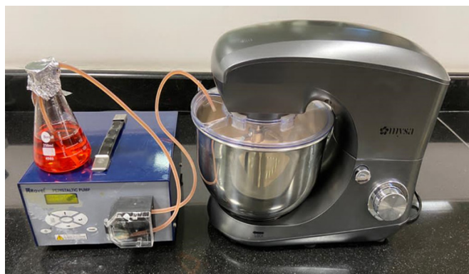
Figure 6. Oil addition with a peristaltic pump for loading with a planetary mixer (MYSA SM-1502 stand mixer by Classique Elements LLP)
