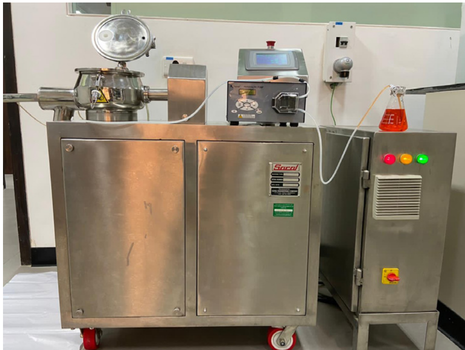
Figure 3. Setup for vitamin E loading into SYLOID® XDP 3150 silica using a rapid mixer granulator (RMG-3L, by Saral Engineering company)
