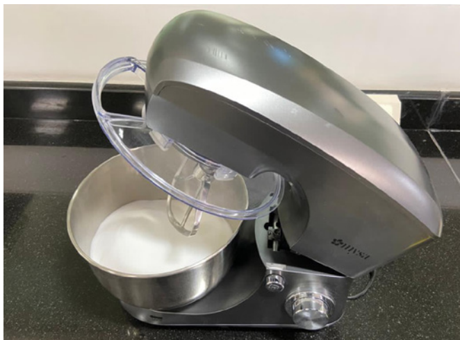
Figure 4. Planetary mixer with SYLOID® XDP 3150 silica in the mixing bowl (MYSA SM-1502 stand mixer by Classique Elements LLP)
