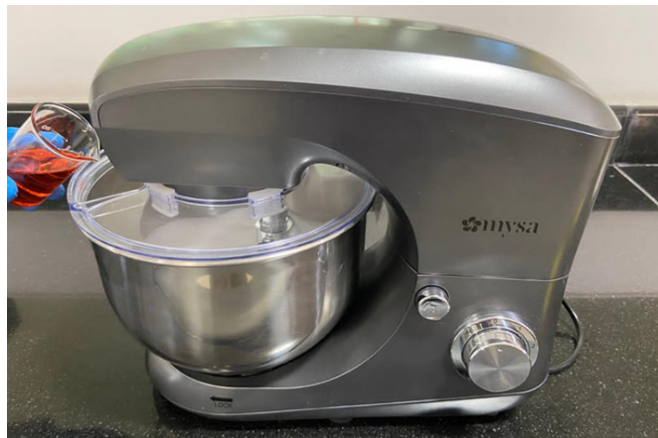
Figure 5. Manual oil addition for loading with a planetary mixer (MYSA SM-1502 stand mixer by Classique Elements LLP)
