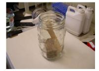
Place your wood pieces in a container and weight them down to prevent floating. The container should be tall enough to prevent foaming over the sides during stabilization.
