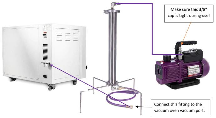
The hose connections are important, we want to make sure our vacuum pump is connected to the top of the column. In any event that excess moisture collects in the column we will avoid gravity draining any trapped water or condensed water vapor from being vacuumed into the pump.
