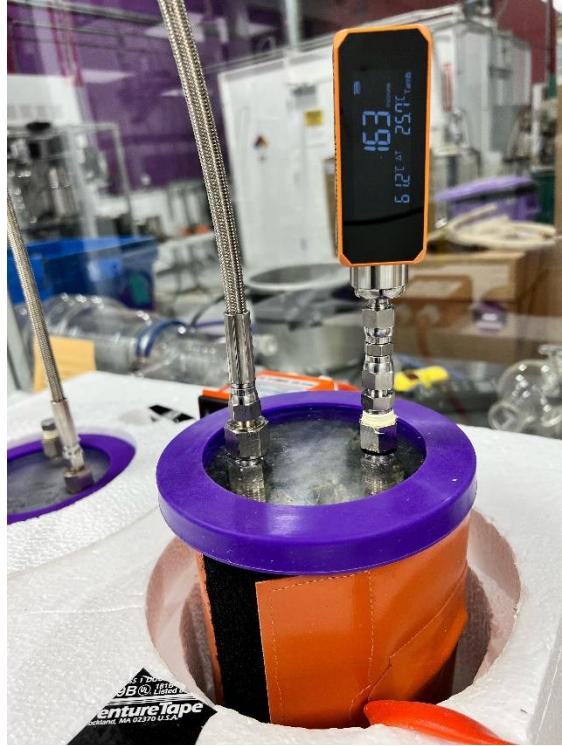
Image 11: Vacuum Gauge Reading Under 300 Microns
