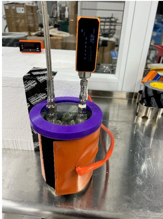
Image 3: Drying Chamber on Flat Surface
