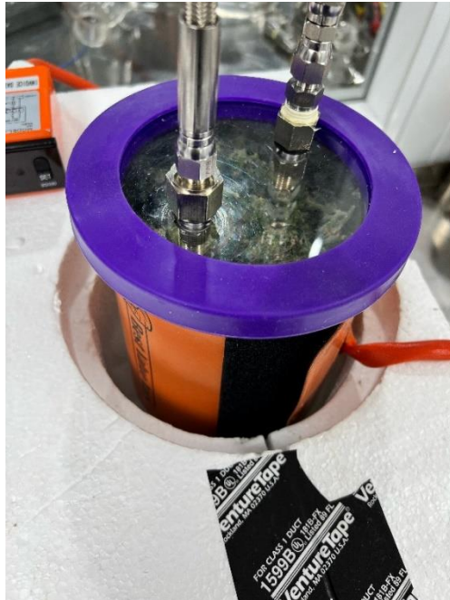
Image 9: Drying Chamber on Top of Dry Ice
