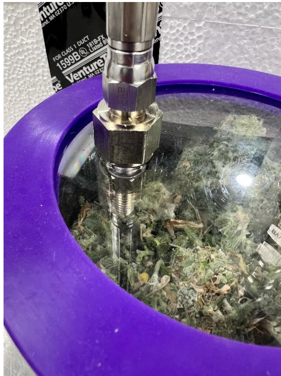
Image 5: Drying Chamber Filled with Biomass
