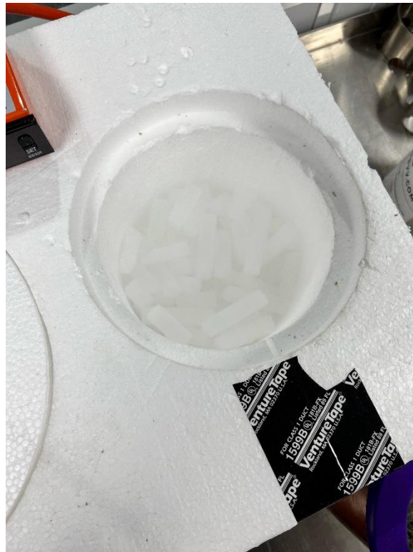
Image 8: Drying Chamber Slot with Dry Ice
