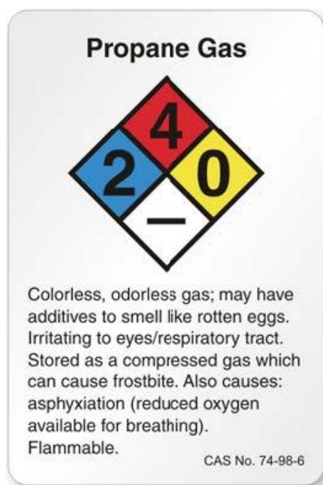
Figure 1 : Sample Propane Warning Label (Right to Know Label) Figure 2 : Sample Propane NFPA 704 Hazard Rating Placard
