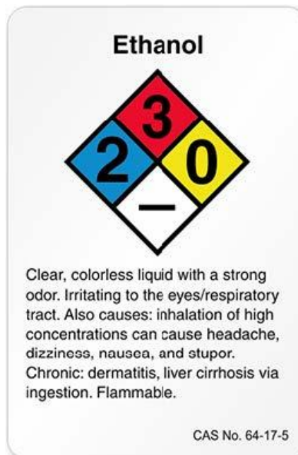
Figure 14 : Sample Ethanol NFPA 704 Hazard Rating Placard
