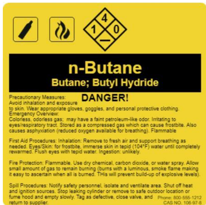
Figure 15 : Sample Butane Warning Label (Right to Know Label)
