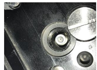
11. Using a plastic tube, push down on the Suction Valve Spring Washer to expose the groove at the top of the Suction Valve Spring.
