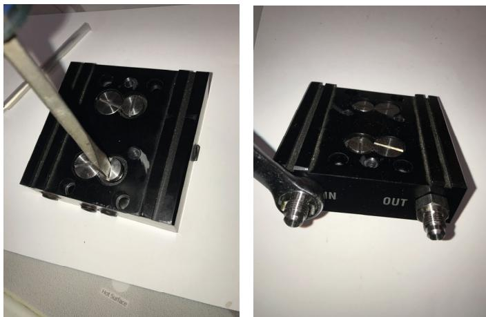
15. Install the kit provided Stainless Steel IN and OUT fittings. Lubricate the O-rings on these fittings. Don't forget to re-install the IN filter screen under the IN fitting.
