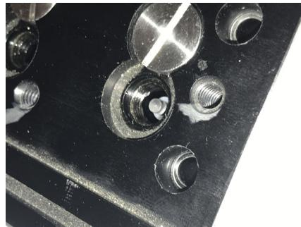
12. Now for the tough part. Stretching the Suction Valve O-ring retainer over the end of the Suction Valve stem onto the groove. The method used below has the O-ring stretched over a small diameter rod. A tubular plastic rod is used to help push the O-ring onto the Suction Valve stem groove.
