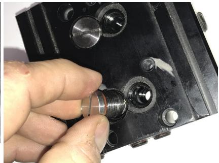
10. Place a suction valve onto its seat. Do one at a time. Once in the seat, flip the head over and place on flat surface to keep the Suction Valve in place. Install Suction Spring onto Suction Valve stem. Install Suction Valve Spring Washer onto Suction Valve stem.
