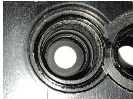
9. Install new discharge valves into the respective cavities. Place Spring onto discharge valve stem. Install the kit provided stainless steel Discharge Valve Covers. Lubricate the O-rings on these covers.
