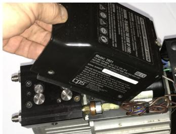
2. Remove the five #2 Phillips head screws on electrical box, remove e-box cover.
