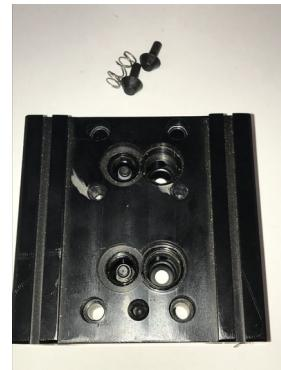
6. Remove the Discharge valves and springs. Discard these.
