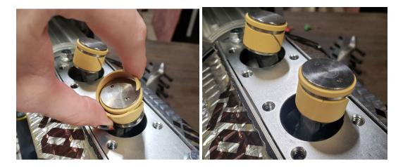
9. Install the matched cylinders and shims over the pistons. The cylinder and shims must go back in the same location. (IMPORTANT: Make sure cylinder walls are free of blemishes and hard resin formations) The piston seals are new and will be very tight when installing the cylinders. Work the cylinder back and forth around the piston top until you can push the cylinders down all the way to the top plate.
