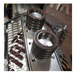
10. Re-install the compressor head onto the top of the cylinders. Hand tightens the compressor head bolts to ensure the head is level. Use a torque wrench to 10 ft-lbf to complete the installation.
