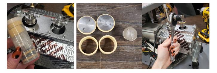
Apply one small drop of Loctite 242 onto exposed threads on the piston base. Install the new Piston Top assembly hand tight onto new Piston Base. Use Piston Wrench to complete tightening with a torque of 2-3 ft.-lbs. Repeat for remaining piston(s).
