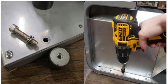
2. Remove the eight 3/16" socket head bolts to remove the compressor head.
