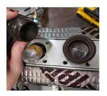
4. Remove and discard Wear Bands. Use Vice Grips to remove Piston Top/Seal assembly. Once the Top Piston assembly has been removed, inspect exposed threads on Piston Base. Clean off any loose dried Loctite from the threads. Wipe the area around the openings clean.
