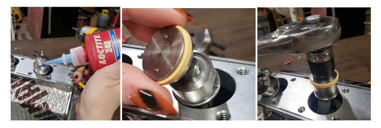
8. Install new Piston Wear Bands on each piston.
