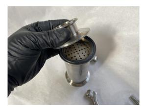
Install another 2.5"->1.5" cap reducer onto the top of the filter housing using the filter itself as the gasket. Tighten bolts to **10ft/lbs**.
