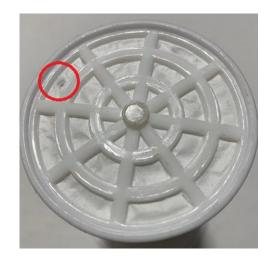
3. *(Optional):* For best results poke a small hole in the filter lid and place in a vacuum oven at 100°F for 30-60 minutes prior to use. This helps eliminate any humidity/moisture that may have accumulated in the media.
