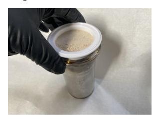
6. Using a seal/bearing punch (available at most automotive stores/harbor freight) firmly press the filter media to ensure a tight packing in case pack was disrupted during the shipping process.
