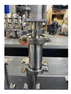
\*Please note, inline housings are not equipped with pressure relief valves or other safety related components. Please ensure your system has adequate protection for where housing is located. Do not place between two ball valves or closed cylinders without adequate protection.
