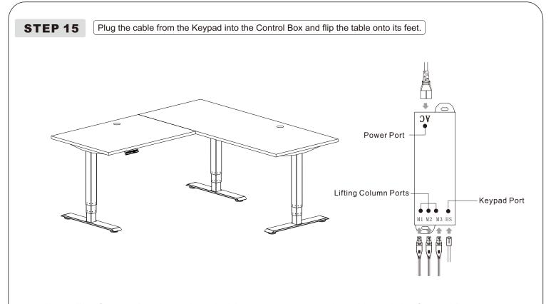
Note: The Control Box is equipped with a gyro sensor so the table and the Control Box must be level in order to work properly or else it will not move up and down.
