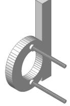
Installation - Fold here & use 1:1 template to mark holes for drilling.
