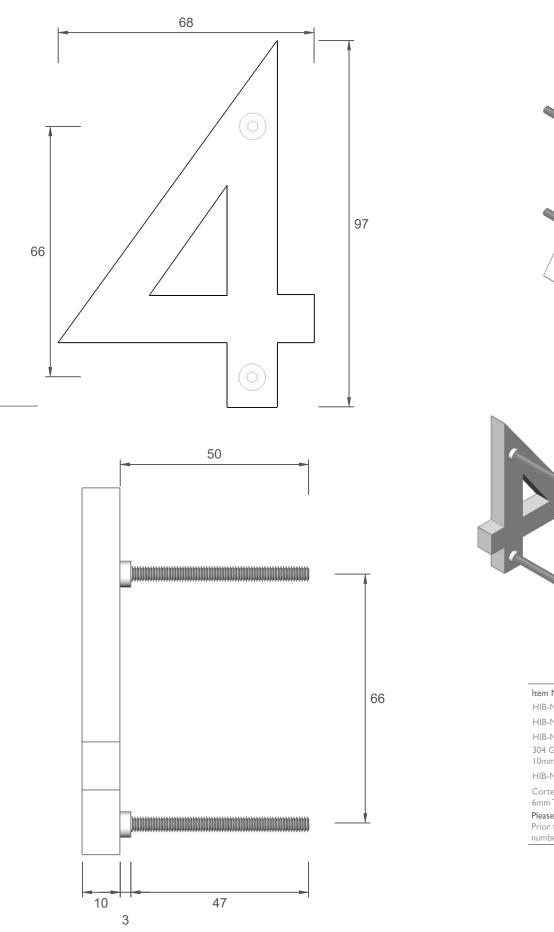
Item Number Finish HIB-N4-SS Brushed Stainless Steel HIB-N4-WHI Powdercoated White HIB-N4-BLK Powdercoated Black 304 Grade Stainless Steel Plate - Laser Cut 10mm Thickness - Solid HIB-N4-CS Rusted Corten Steel Plate - Laser Cut 6mm Thickness - Solid Please note: Dimensions are subject to change. Prior to installation the dimensions on the actual number, or letter, should be checked.
