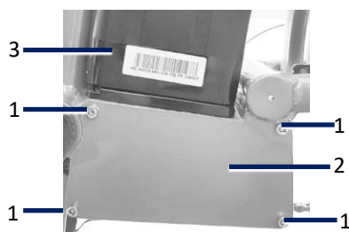
Figure UT1. The controller cover is located on the left side of the bike, underneath the battery (3). Remove battery, remove the four bolts (1), remove controller cover plate (2) to access the controller.
