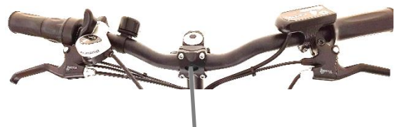
Figure FS3: View from front: Fasten all bolts which hold handle-bar (4 bolts shown in picture) to 18 Nm
