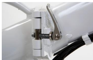
A) quick release lever in firmly closed position
