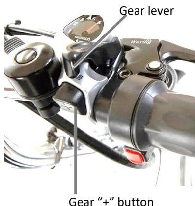
Figure G1: Parts of gear shifter
