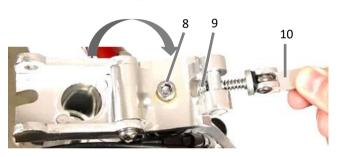
**Figure QF4:** view from top, folded handle-stem. While pushing **quick release lever (10)** down, carefully **fold stem UP in the direction shown until it's fully closed.** For twist-release refer to Figure QF9.
