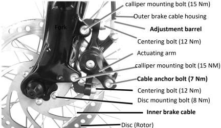
Figure DB1: Disc Brake Assembly: View from left side
