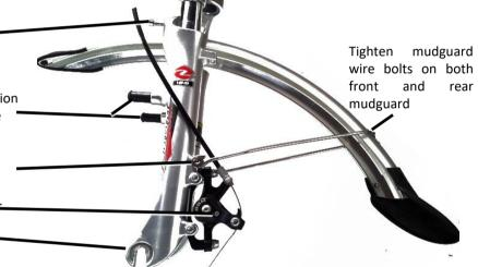
Ensure all parts of the front and rear mudguards and wires have at least 6mm clearance from the tire and wheel. **WARNING:** If the front and rear mudguards are not correctly installed they may prevent the wheel from spinning or turning while riding and cause serious injury. Check tightness of all bolts and correct installation every 30 days.
