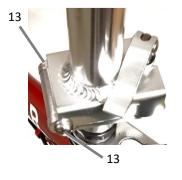
Figure QF6: view from top. Close the quick-release lever as shown. Check that the stem is stable and safely closed. If the stem is loose you may have to tighten the quick release nut (9, Figure QF4) or the hinge bolts (13)
