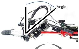
Figure BQ1: view from top. Handle-stem is folded to the right side of bike. Note the angle of about 40 degrees.
