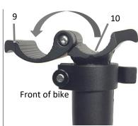
of handle-bar. Top of handle-stem. Open top bracket (9). Insert the centre of the handle-bar into the lower bracket (10). Close the top bracket (9). Install the quick-release mechanism (Figure BQ5), tighten the quick-release nut (6, Figure BQ5) and close the quick
