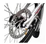
3) Carefully place front wheel threads fully into fork. Make sure the disc goes between the two brake pads of the disc brake.
