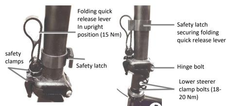
2) Ensure safety clamps are closed, move quick release lever into an upright position.
