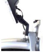
Install front light on top part of fork using bolt (and nut if your model has nut) as shown in the picture above. The bolt of some forks is attached to rear facing part of fork.
