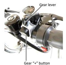
Figure G1: Parts of gear shifter
