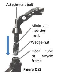
Figure QS1-3: Parts of the quill-type handlestem.
