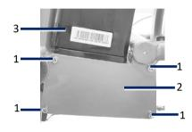
Figure UT1. The controller cover is located on the left side of the bike, underneath the battery (3). Remove battery, remove the four bolts (1), remove controller cover plate (2) to access the controller.
