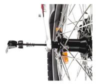
5) Insert skewer. Sometimes there may be plastic residues inside the hole which need to be pushed out with the skewer. Don't use extreme force.
