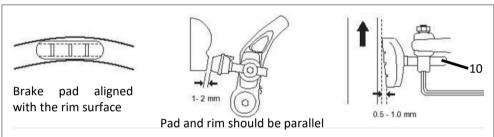
**Figure RB1: Right:** large arrow shows direction of rim rotation. Brakes should be "toed-in" so the rear portion of each brake pad is about 0.5-1mm farther from the rim than the front portion of the brake pad
