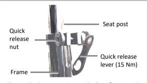
**Figure S2**: Seat post is attached to frame with quick-release mechanism.
