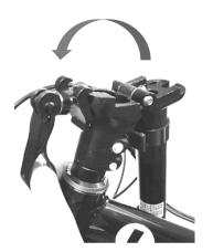
1) While pulling quick release lever down, carefully fold stem UP until it's fully closed
