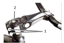
Figure DS1: The steerer clamp bolts (1) attach the stem to the bike. To adjust the alignment of the stem with the front wheel, loosen steerer clamp bolts (1) and tighten after alignment to 13 Nm. Make sure the centre bolt (2) is tight (13 Nm). Direct connect stems cannot be adjusted in height.
