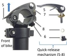
Figure BQ5. Installation of handle-bar. Top of handle-stem. Open quick-release lever (5). Unscrew quick-release nut (6) and remove the quick-release mechanism including top washer (7) and bottom washer (8).
