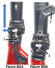
side. Quick release lever (1) is open. Move the quick release lever (1) left to unlock it, then up to close it.
