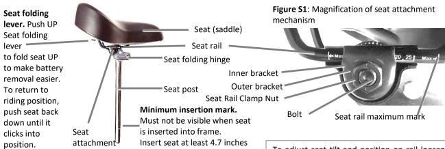
The model SuperT does NOT have a folding seat post. The seat needs to be twisted to remove the battery.
