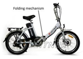
3) The folding frame is now straight. Follow the guide below to lock the frame safely before riding. The handle-bar can be straightened later. First lock the frame.
