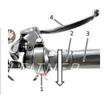
Figure C1: The twist-and-go throttle (2) is located on the right hand side of the handlebar, next to the handlegrip (3). Push the red button (1) IN to switch the throttle on. Push the red button (1) again, so that it moves OUT to disable throttle.
