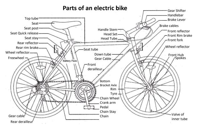
Figure B1: Parts of an electric bike. Some parts may not be on your model.
