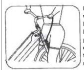
Figure BQ8: To align stem with wheel, walk to front of bike, put wheel between your legs and adjust handle-stem position. Tighten lower steerer clamp bolts (12, Figure BQ9) to 18-20 Nm. If needed first release lower steerer clamp
