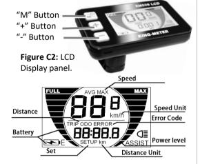
**Figure C3:** Screen of LCD Display panel. If error code is displayed stop riding bike and contact customer service at sales@leitner.com.au
