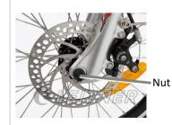
7) Insert one spring onto skewer on this side and fasten nut onto the threads on the end of the skewer by hand. Close the quick release lever on the other side. Refer to the section "Quick Release Levers" of this manual to ensure correct use.
