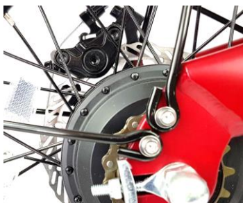
Figure M5: Correctly attached wires to frame. (Right side of bike).
