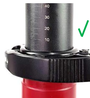
Figure B3: Minimum Insertion Mark NOT Visible. CORRECT.
