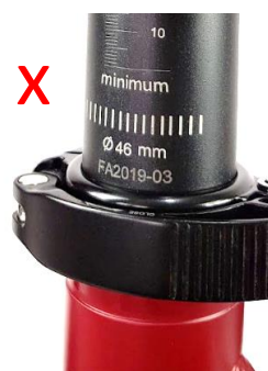
Figure B2: Minimum Insertion Mark visible. NOT CORRECT.
