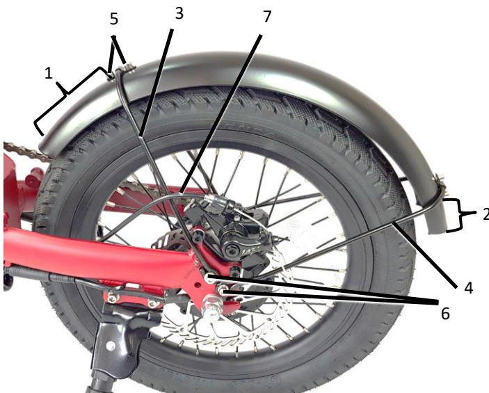
Figure M3: Left: Correctly attached wire to mudguard (view from top). Use two small bolts (5) with 5mm thread length, black washer (8) . Right: View from bottom. Use silver washer (9) at bottom.
