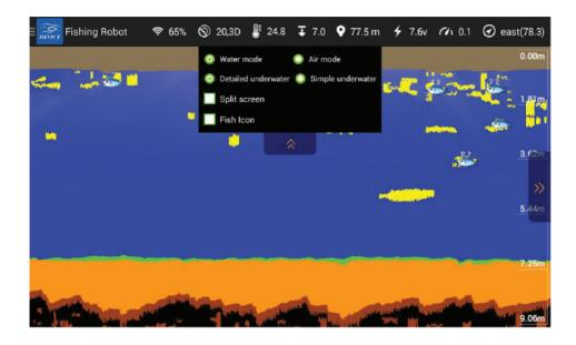
The sonar detection displays from right to left. The right side of the screen is your boats current location in the water.
