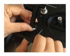
To attach the device holder to the handset, remove the small hexheaded bolt and nut from the bottom of the mounting arm.
