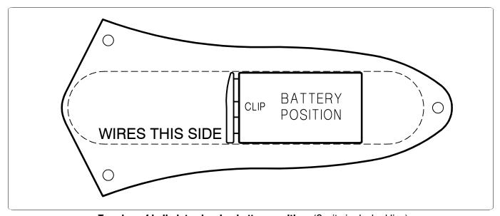
**Top view of bell plate showing battery position** (Cavity in dashed line)
