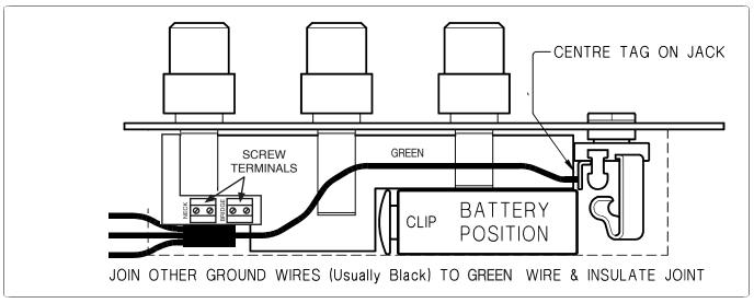
Side view of the J-RETRO in the bass showing connections (Cavity in dashed line)
