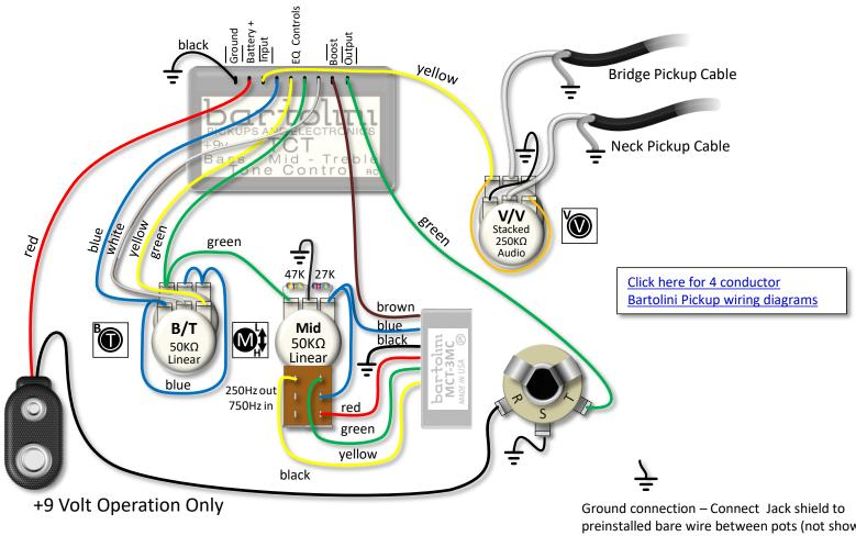
Ground connection – Connect Jack shield to preinstalled bare wire between pots (not shown in this diagram). Connect to cavity shield if available. Also ensure bridge is connected to ground.
